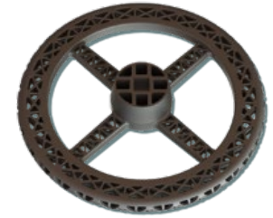
Component designed with lattice structure
