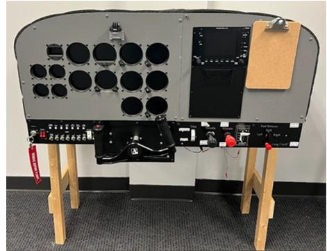
ODU’s Office of Enterprise Research and Innovation possessed the Cessna 172 control panel simulator. It was constructed for a previous project but was no longer being used. The Academy was excited to receive it. The simulator can provide students with basic knowledge and skills of how to fly a Cessna 172 and likely expand their interest in the world of aviation.
