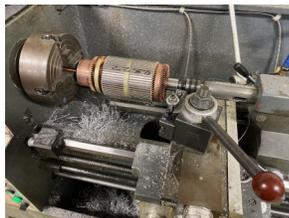
Turning down shaft diameter to fit a standard ball bearing
